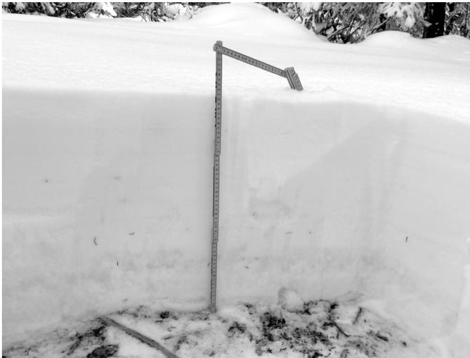
Figure B.3. Folding rule placed against pit wall for measurement height reference. It is often easier to secure a folding rule than a probe section by folding the unused portion and gently inserting it into the snow surface in a location that will not interfere with other measurements. If snowpits are deeper than 2 m, a probe is preferable and may be secured against the pit wall with small sticks or snow. Remove any unneeded sections to minimize tipping by wind.
