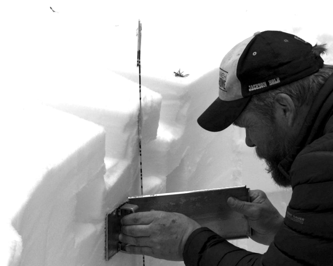
Figure B.6. Hold the sample in the pit wall with one hand while inserting the lid with the other. Angle of insertion is important for the lid to avoid sample error.
