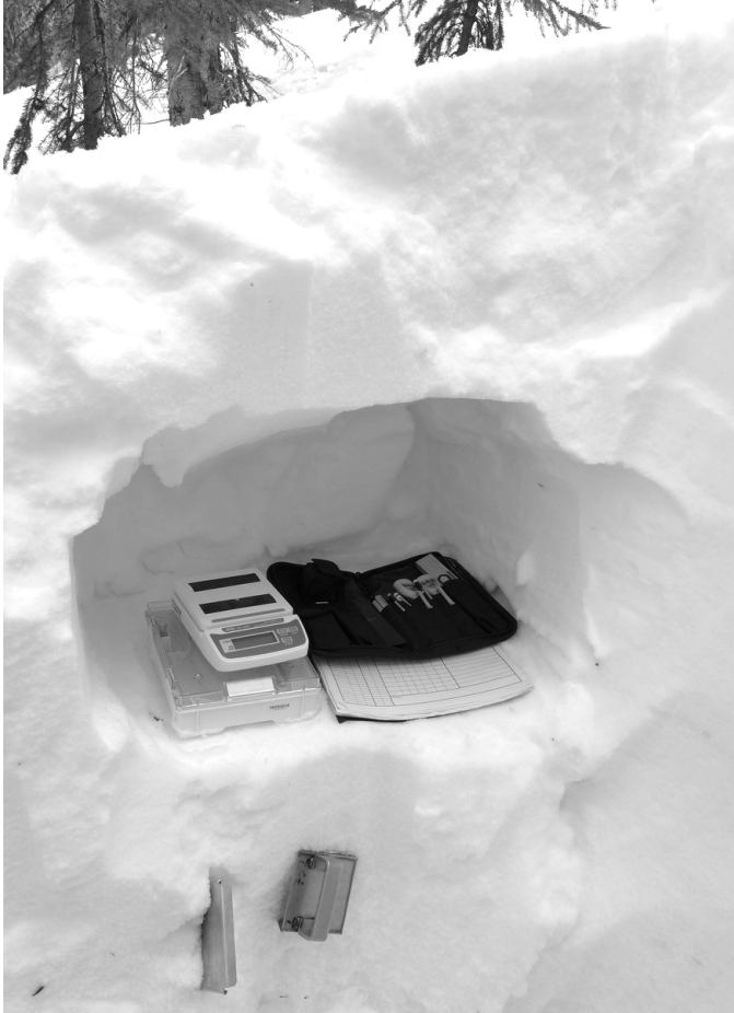
Figure B.4. Excavated hole in snowpit flank to provide a flat, protected location for the scale and fieldbook. Note that there is plenty of room to bring the density sampler in and out of the hole without knocking snow onto the scale or notebook. If the hole is too big, blowing snow will accumulate on the scale and book.
