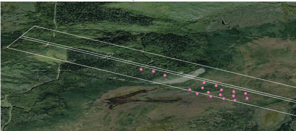
Figure. Example layout of SWESARR flight lines and corner reflector locations (to be updated after CR locations are finalized).
