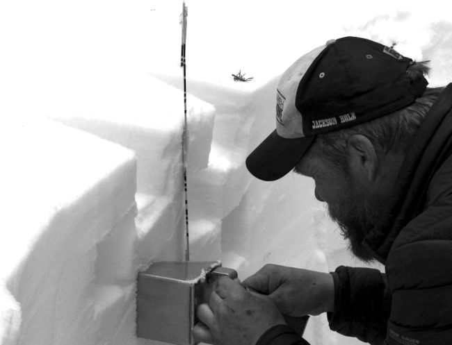
Figure B.5. Carefully line the sampler up so the back plate is parallel to the pit face in all directions when fully inserted.
