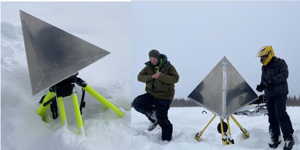
Figure. 18" (left) and 36" (right) corner reflectors deployed in BCEF as part of a March 2022 experiment.
